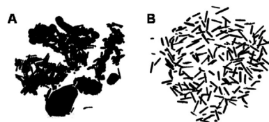
Figure 4. Unique intracellular distribution of tannic acid GNRs. TEM images of (A) TAT HA2 GNRs and (B) TA GNRs were converted to binary images to assess the spatial orientation of aspect ratio 6 GNRs within HaCaT cells. From these results, the particle area fractions were determined in order to evaluate the preservation of GNR particle integrity. With TA functionalization, nanorod morphology is maintained, whereas GNRs were found to fuse together with TAT HA2 surface coating.
